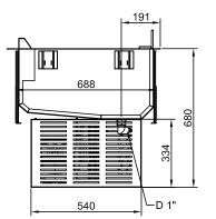
Drain Electrical inlet (power)
